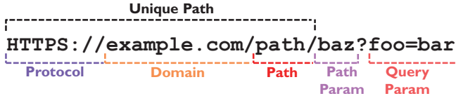
Fig. 2: Structure of a URL for example.com. Typically, parameters can be sent both in the URL and in the body of the HTTP request. We ignore the parameters to find the unique paths.
